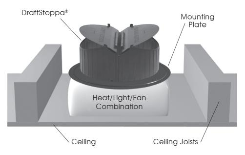
**WARNING:** When installing a DraftStoppa® over Heat/Light/Fan combination units, the switch must be rewired by a qualified electrician in accordance with the AS/ NZS 3000:2007 wiring instructions to ensure the <u>fan always operates when the heat lamps are in use</u>. Detailed information included with DraftStoppa® instructions.
